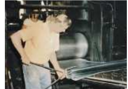
Fig. 2: The pack-rolling process for sheet metal was used until the 1960s in Central Europe and is still used in some parts of Eastern Europe.
